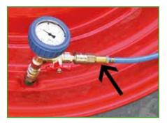
The PTG valve is screwed into the tyre valve after the valve core has been removed (increased air flow).
