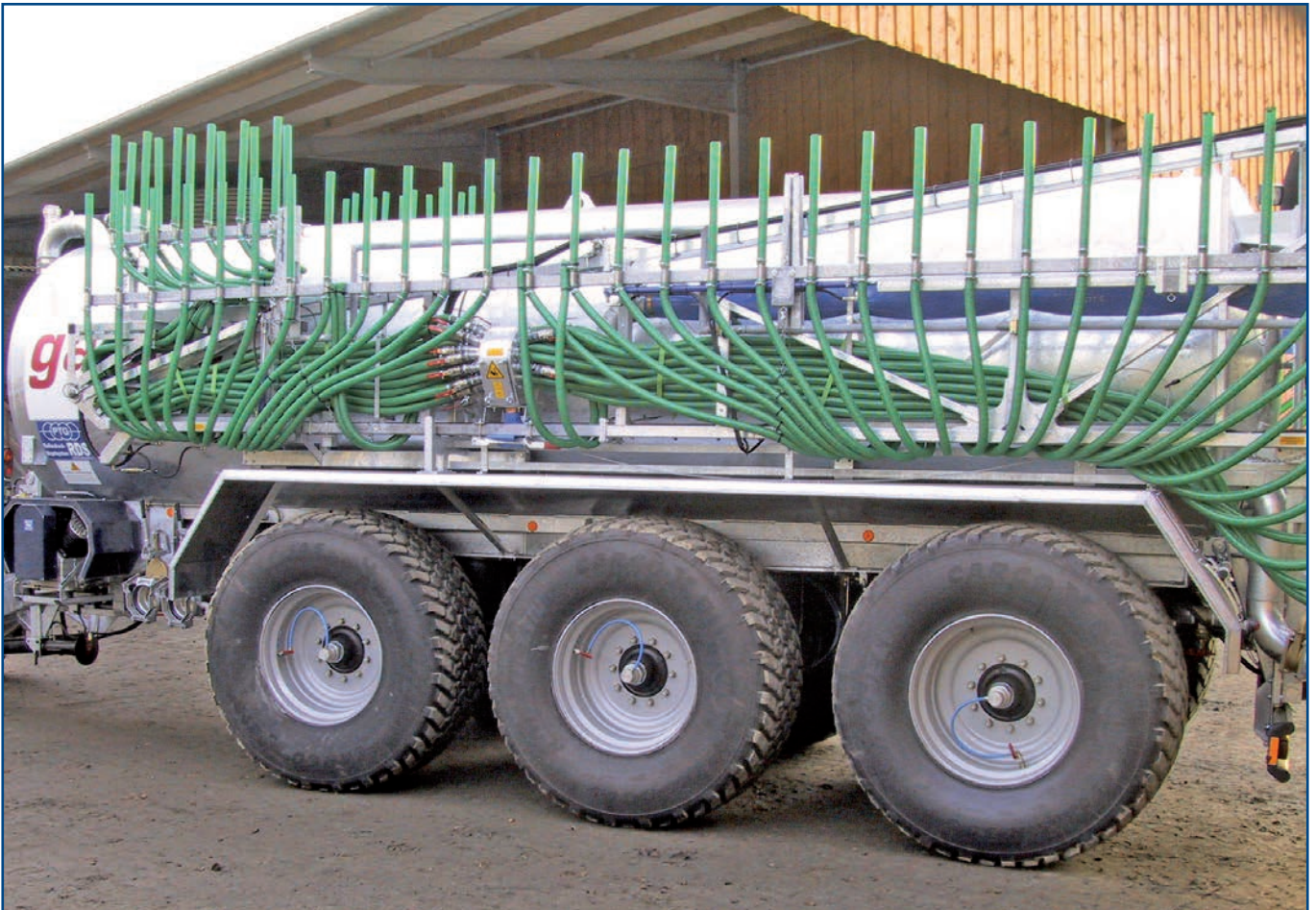
RDS 1L with pneumatic control Single line tyre inflation system for slurry tankers & trailers
