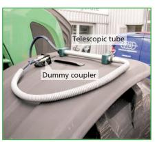
The air and control lines are connected to the rotary unions with special quick connectors, so the lines can be disconnected easily when not in use and kept in dummy couplers on the mudquards.
