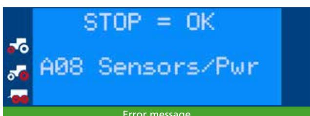
After rectifying the error, to resume full use of the central tire inflation system, it is necessary to switch it off and on again. To acknowledge the error, the operating console must be switched off and on again using the toggle switch.
